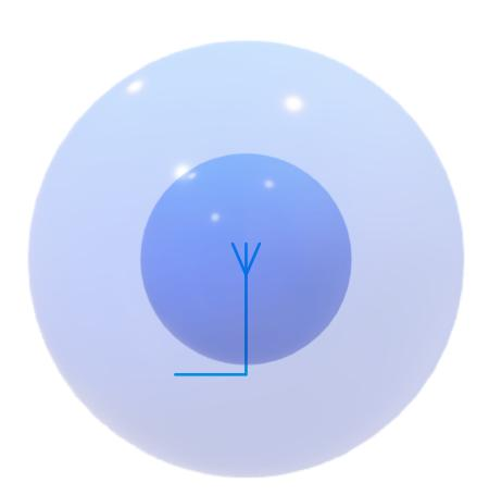
An **isotropic** antenna radiates a perfect sphere
