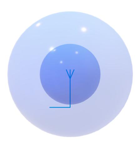
The size of an isotropic antenna is related to wavelength
