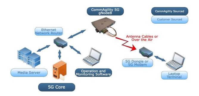
The 5G Reference gNodeB is a preintegrated system, including both hardware and software, and is based on the NXP Layerscape® Access® 5G integrated SoC chipset.
