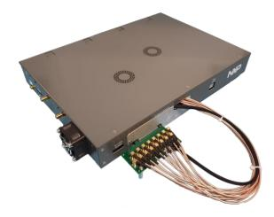
The LA1224-RDB is an NXP development platform featuring an LA1224 Layerscape Access fully programmable baseband SoC. It is coupled with an NXP LX2160A, the highest performance member of the Layerscape multicore communications processor family.
