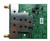
When used in conjunction with the LA1224-RDB, the RF module provides a complete baseband and RF small cell solution with a 2x2 MIMO air interface. RF output power up to +12dBm average is supported (depending on frequency), and bandwidths up to 60MHz on each of two band n78 TDD 3300-3800MHz RF channels (also covers band n48 CBRS TDD 3550-3700MHz).
